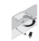
Push swing arm clockwise until it locks in to place, firmly holding the blind headrail.
