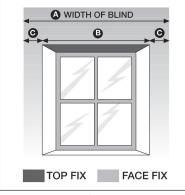
Place blind in fitting position. Space the brackets evenly. Leave 3cm clearance at either end of the rail to prevent interference with side winder mechanism.
